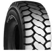
Deep tread pattern with sidewall protectors. Specifically designed for giant dump trucks. Non-directional deep tread pattern ensures excellent traction and strong resistance to side-slipping as well as long life and cut resistance on rocky surfaces.
