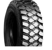
Provides good traction, generates low heat and assures long tread life on soft, muddy or packed surfaces.
