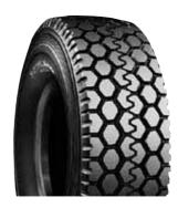
VSB exhibits excellent traction and maneuverability. Suitable for both gravel and hard packed surfaces like paved roads. Designed for heavy-duty trucks and trailers.
