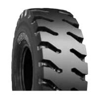
Extra super deep tread designed for severe or rocky surfaces, offering excellent traction, stability and a comfortable ride. Specially designed sidewall provides extended protection from cutting. For use in underground mines, open pits and quarries.
