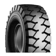
Extra-thick tread pattern VRQP assures longer tread life and superior cut resistance. Greatly reduces total tire costs for replacement. Specially developed for mid-size rigid dump trucks working in quarries and other tough operations.
