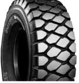
Normal-depth tread with a nondirectional traction pattern, featuring strong resistance to heat buildup. Most suitable for hauling equipment used in coal mines, and equally applicable to operations on soft or muddy surfaces.
