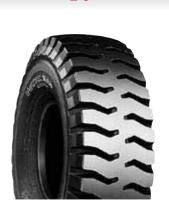
Normal-depth tread designed for longer and higher speed hauling. VRL's attributes, including great resistance to heat build-up, and strong resistance to cutting and chipping, make it suitable for large dump trucks in earthmoving work.
