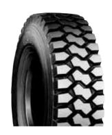
This tire's features are extra-long life, superior cut resistance and excellent traction. The casing is reinforced by  $\star 3$  for heavy-duty mining trucks in cyclical operation.
