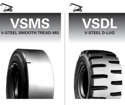
Smooth extra-deep tread with a reinforced all-steel radial casing. For container handling equipment especially on abrasive concrete surfaces.
