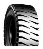
Normal-depth tread with sidewall protectors. High resistance to shock damage, cutting and chipping. Suitable for rocky surfaces, such as rocky or packed roads.
