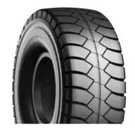
Extra-deep tread pattern with sidewall protectors. VZTP focuses especially on traction, extra-long tread life and superior cut resistance. Narrow center tread grooves, which reduce tread block movement and help with heat dissipation, along with wider side lugs, achieves the perfect balance of opposing performance targets: traction, tread life, and heat resistance. VZTP can be the best solution for large, rigid dump trucks working on muddy surfaces.
