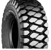
Non-directional deep tread pattern for strong traction, especially resistant to side-slipping. High wear resistance ensures long tread life. Applicable for muddy or soft surfaces.
