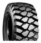
Offers outstanding cut resistance and long tread life on rocky or gravel surfaces in mining, quarry and construction, with superior traction.
