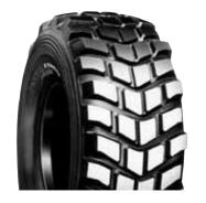
Ideal for soft or muddy surfaces, offering good traction and flotation.
